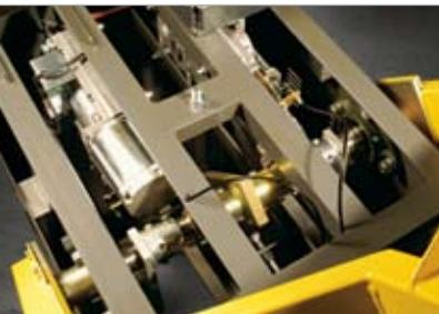
**Double motor, double lasting power.** GARD 12000 is equipped with nothing other than 2 gearmotors, which are installed along the same axis and provide remarkable torque.
